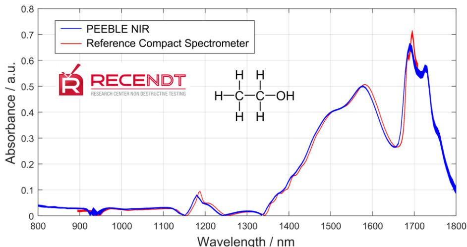
**Figure 3: Absorption of ethanol measured in a quartz-glass cuvette with 1 mm path length.**
