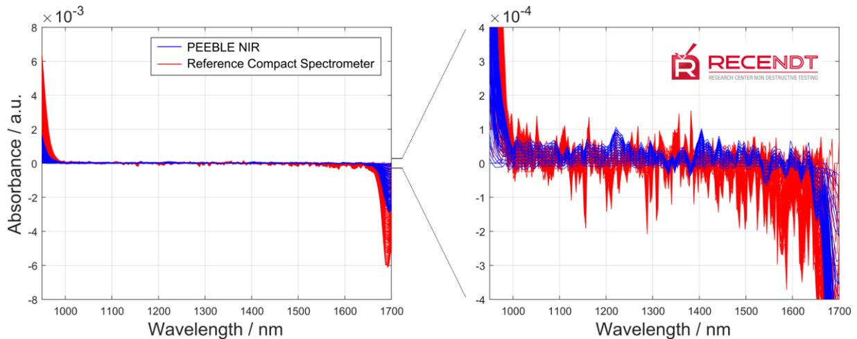
**Figure 2: 100% Lines of the PEEBLE NIR compared to the reference compact spectrometer with similar specifications.**
