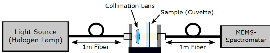
**Figure 1: Schematic drawing of the experimental setup used for the conducted comparison measurements.**
